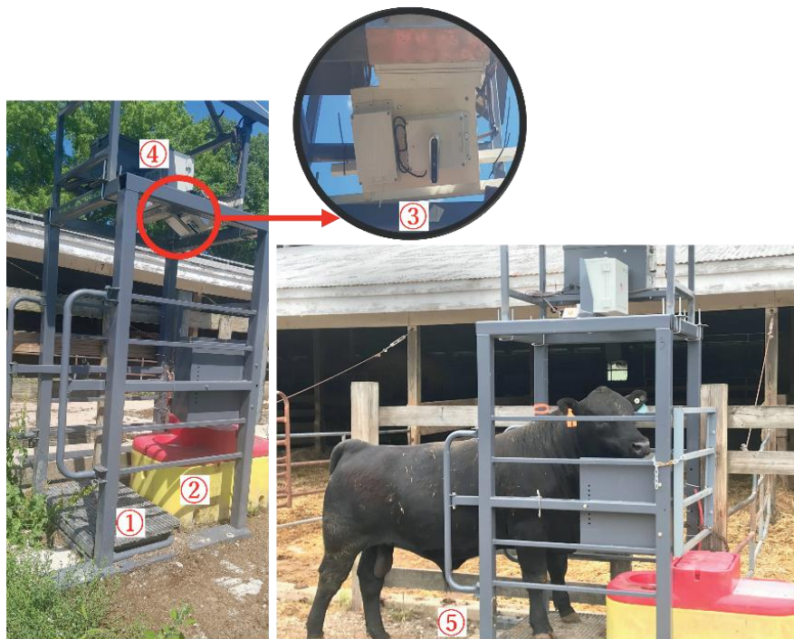
Figure 1: Structure of the vision system: (1) mainframe, (2) waterer, (3) sensing unit, (4) solar panel kit, and (5) animal enter the waterer.
