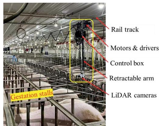
Figure 1: The overview of the developed robotic imaging system.
