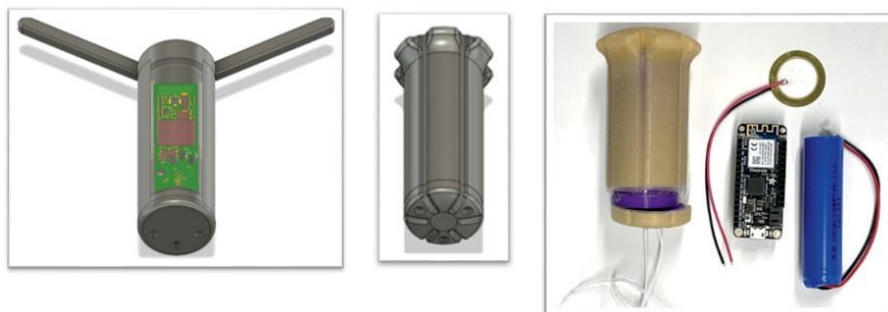
Figure 1: Intravaginal instrumentation device parts and assembly, with the initial hard-shell design and wings on the left, improved hard-shell design in center, and covered with silicone and internal components on the right.
