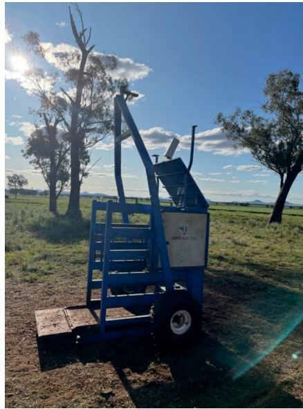
Figure 1: Optiweigh used at Nowley Farm, NSW, measuring cattle liveweight
